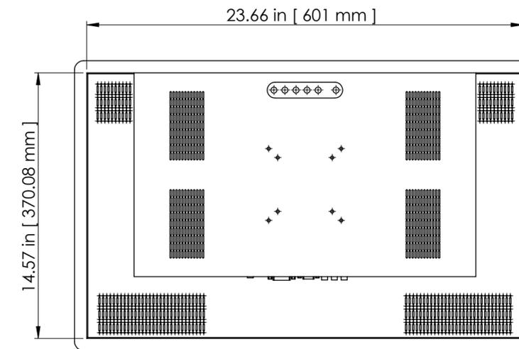
This cutout dimension applies to all different variations of SL-PPC-24A with or without attached "Ebox". If mounting through a panel or a wall, refer to this drawing for proper cutout measurements.
